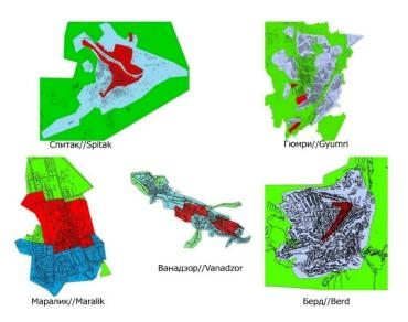
Fig. 2. Maps of seismic risk of damage residential and public buildings in the territory of the cities of Armenia located in intensity zones 1988 Spitak earthquake: Spitak (9-10 points), Gyumri (9), Vanadzor (8-9), Maralik (7), Berd (6-7) [4]. The colors indicate risks level: red - high; blue - average; green – absent.
