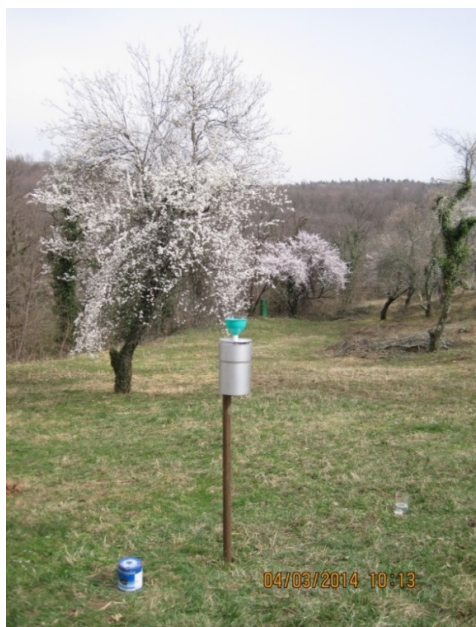
Figure 4 Palmex rain collector (2014/2240 GW84: 42.60105°E 42,37688°N 180m) installed next to the visitor centre of Prometheus Cave ©Foto: M. Kralik
